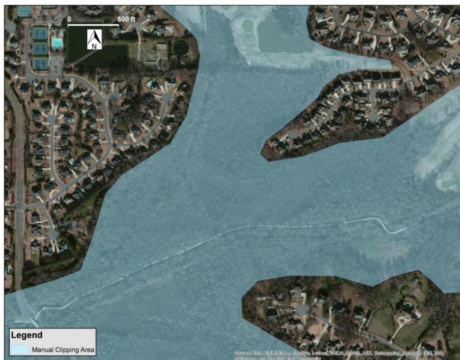
Figure 7–12. Example of a manually digitized polygon where no assets are at risk of flooding (Big Creek subwatershed).
